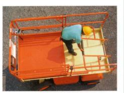
After entering the deck, simply disengage and fold the rear railing down to the deck....
