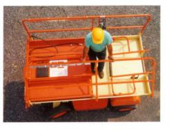
....after front and rear railings are collapsed, main siderails can then be lowered....
