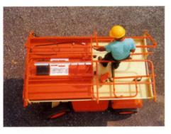
....after folding handrails down, machine height is reduced by 0.8 m (2 ft. 6 in.) and the unit can be driven using its moveable control box and 1.8 m (6 ft.) umbilical cord, enabling travel through standard double doorways.
