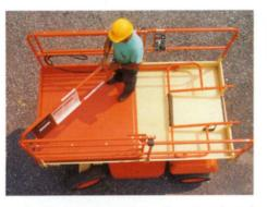
....the front rail is then disengaged and folded in, along the left siderail...
